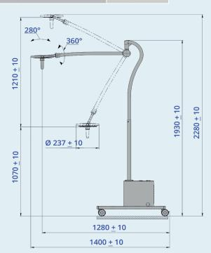
The mobile examination light EMALED 202 M with a battery back-up can be used without power connection up to 24 hours. The high illumination and excellent lightning quality makes this mobile surgical light a good allrounder in multiple fields.
